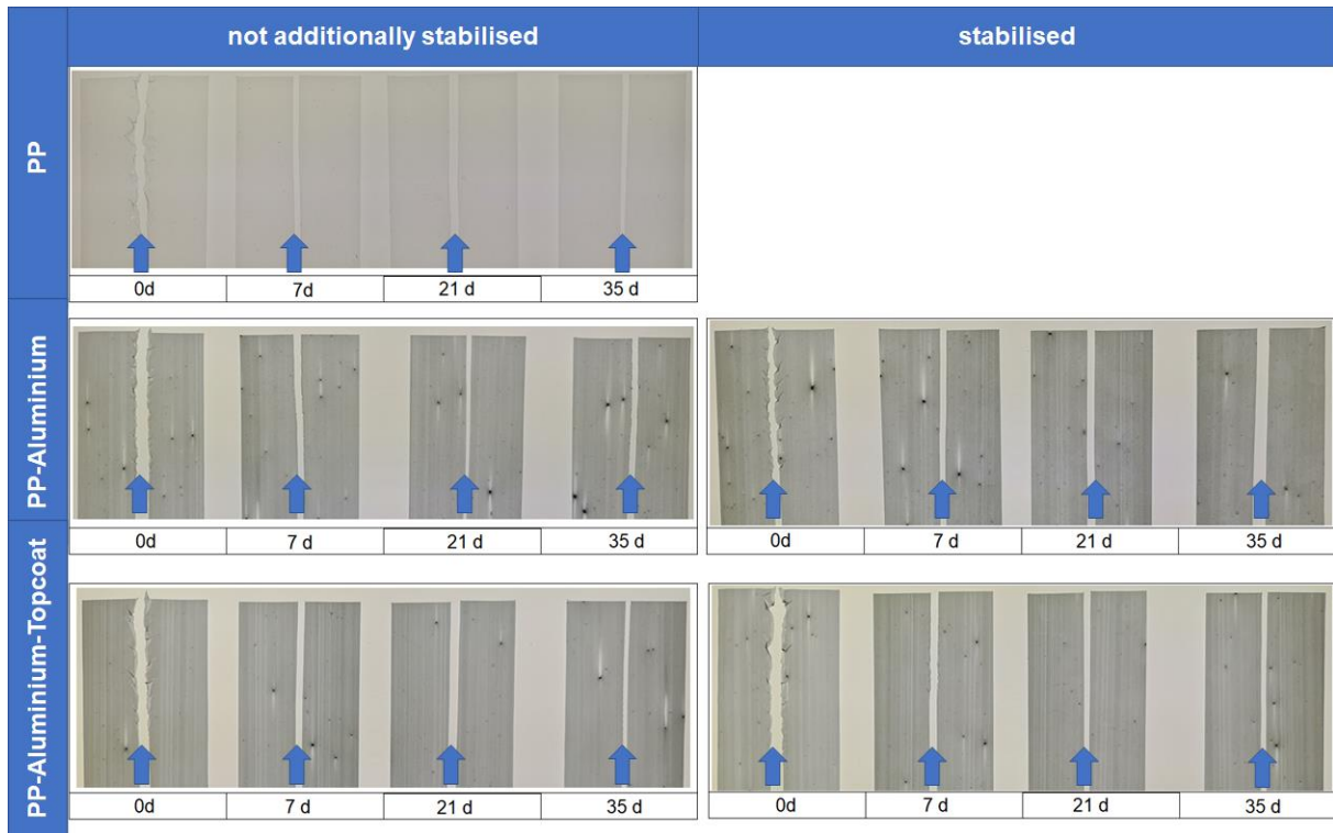
Figure 5: Specimens after tear propagation testing of the different film formulations in the initial condition (0 d) and after different storage times in the convection oven at 100°C (arrow marks the beginning & direction of the tear).
